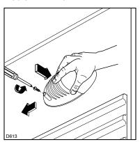
Unscrew the light cover and then pull it outward by pressing as shown in the figure. Unscrew the bulb and replace it with a new 15 watt bulb (available from your nearest Service Force Centre).
